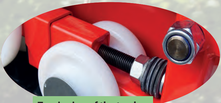
Tensioning of the tracks with a standard tool
