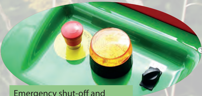
Emergency shut-off and LED signal lighting for safety
